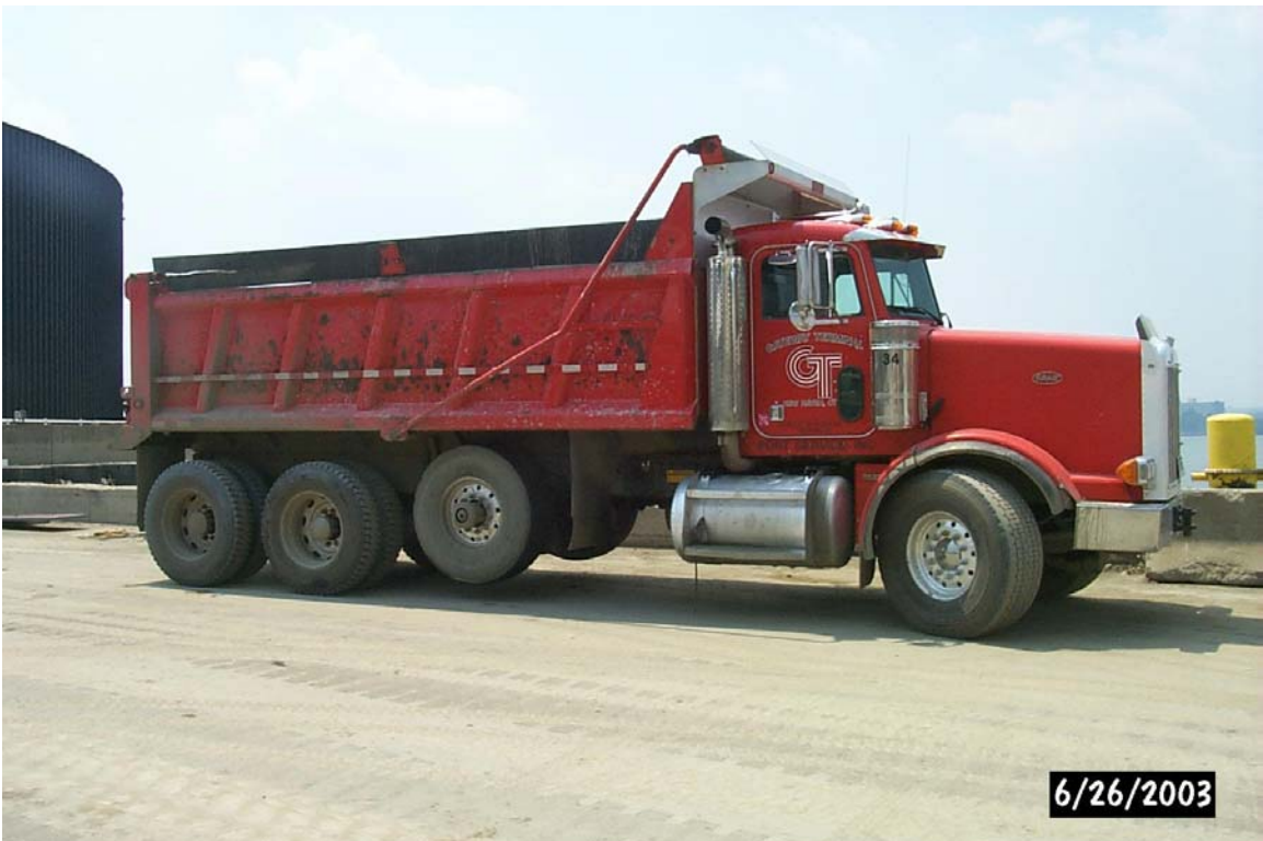
2000 Peterbilt model 357 tri-axle dump truck. Steel body with electric tarp and air tail gate. Caterpillar C-12, 410 hp with Eaton Auto Stick 18 speed trans. excellent rubber on all axles. Truck runs excellent and has service records available upon request. Ready to go to work
